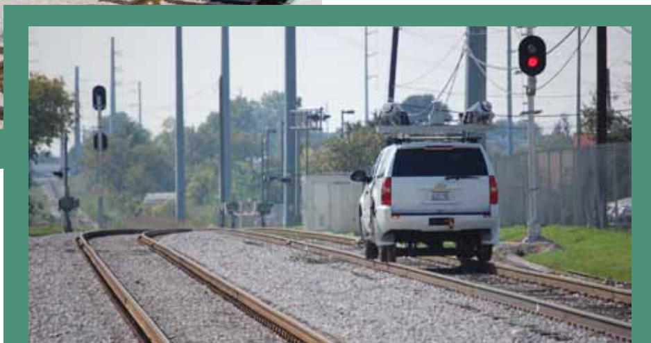
Left: The SAM mobile LiDAR hi-rail vehicle travels through a commuter station during its first full rail project. Below: The mobile LiDAR unit scans a section of railway, also picking up transmission lines along the track right-of-way.
